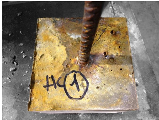
(a) CC concrete at 1.6% corrosion level
