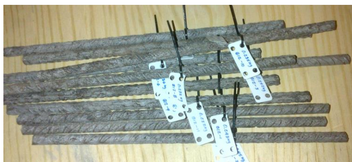
Figure V-24. Statically-undetermined beams. Cleaned specimens
