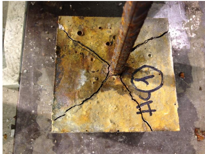
Figure IV-22. Specimen after pull-out test
