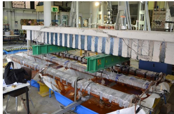
Figure III-3. Test configuration during corrosion procedure
