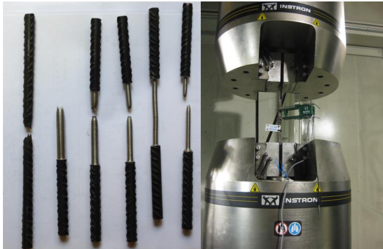
Figure V-1. a) Reduced cross-section specimens. b) INSTRON 8800 transducer
