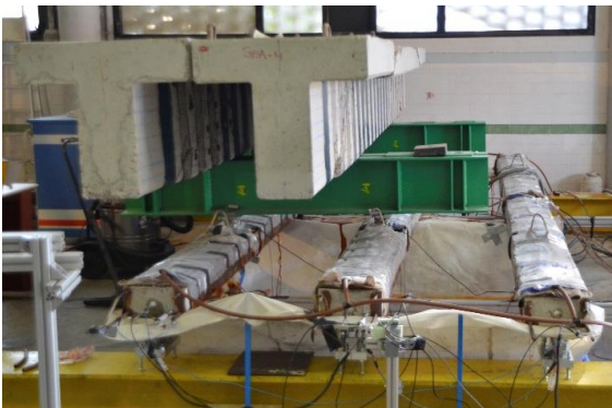
Figure III-3. Test configuration during corrosion procedure
