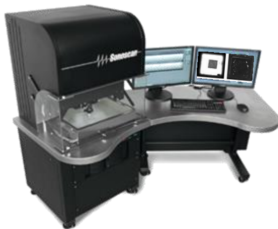
Figure 3.2. Sonoscan GEN-5 SAM system used for die-attach analysis.
