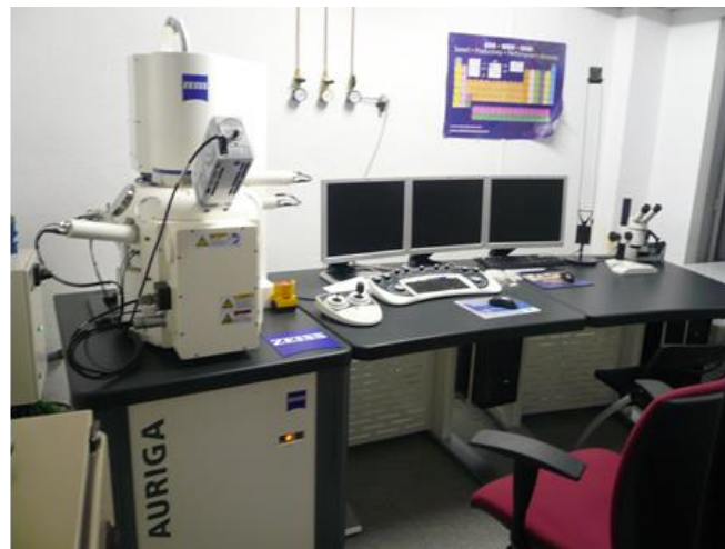
Figure 3.6. Carl Zeiss Auriga 40 SEM-EDX workstation used for die-attach layer analysis.
