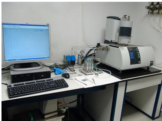
Figure 3.12. NETZSCH STA 449 F1 Jupiter TGA/DTA system used to characterize Ag pastes.
