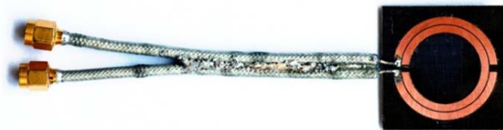
Figure 5.4. SRR antenna input impedance measurement assembly.
