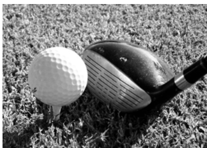
Figure 2.10. Polyurethane ionomer cover of golf balls provides hardness, abrasion resistance and durability.
