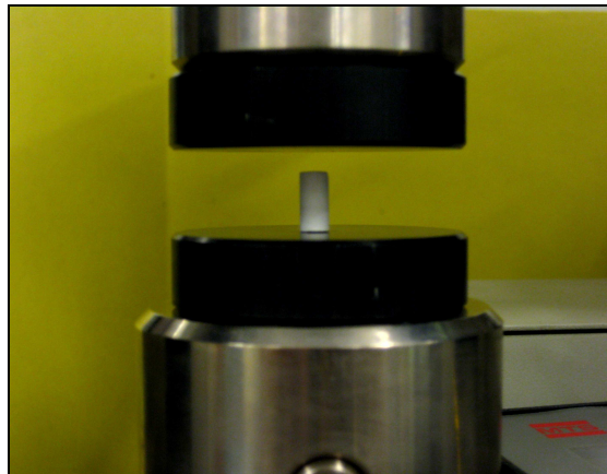
Figure 1.4. Cements are tested under compression in an electromechanical testing machine. The maximum compressive strength at failure is recorded against the reaction time to obtain the hardening curve, i.e. C(x_i, t) .
