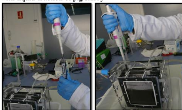
Figure 3.7. Biofilm sampling from the MFC fed with synthetic medium. The graphite granules sample was taken from the anode to inoculate anode material/chamber in MFC fed with liquid fraction of pig slurry.
