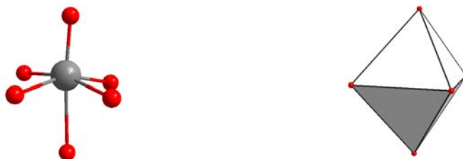
Figure 3.1. Ball-and-stick (left) and polyhedral (right) representation of the fundamental \text{MO}_6 unit. Colors for the atoms: O, red; W, grey.
