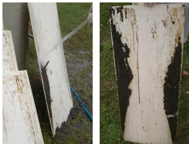
Figure 6.5. Images of cake formation on the membranes due to insufficient aeration.
