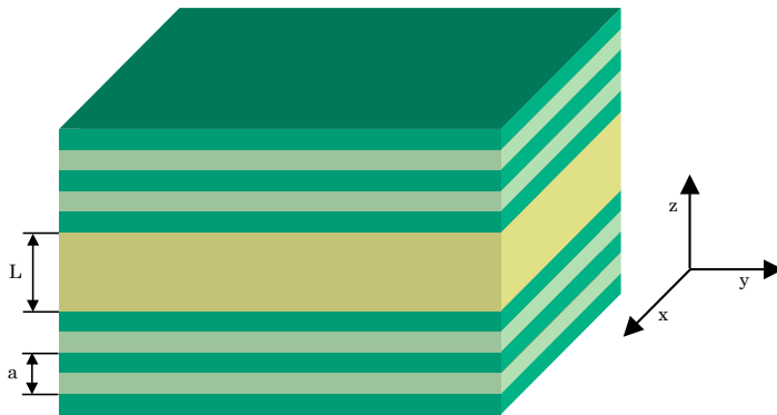
Figure 7.19. Schematic illustration of a photonic crystal with a defect, or microcavity. Defect modes appearing in such structure will be localized near the different colored layer that breaks the symmetry in the z-direction.
