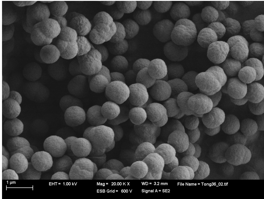
Figure 4.10. SEM of M36-02 prepared by precipitation polymerization method
