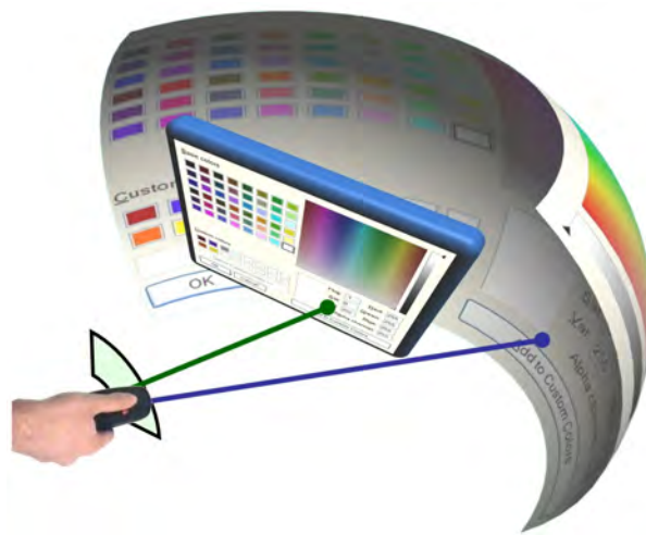
Figure 6.12: Manipulation with friction surfaces simulates approximately the interaction with a large spherical window. Note that rendering this simulated window would be unusable as it would occlude most of the scene.
