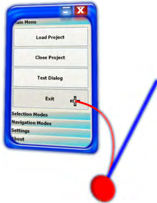
Figure 6.7: The red ray corresponds to the feedback ray and the blue ray to the real device ray. The selection ray is not displayed but its defined by the hand's position and the intersection point between the feedback ray and the virtual window.
