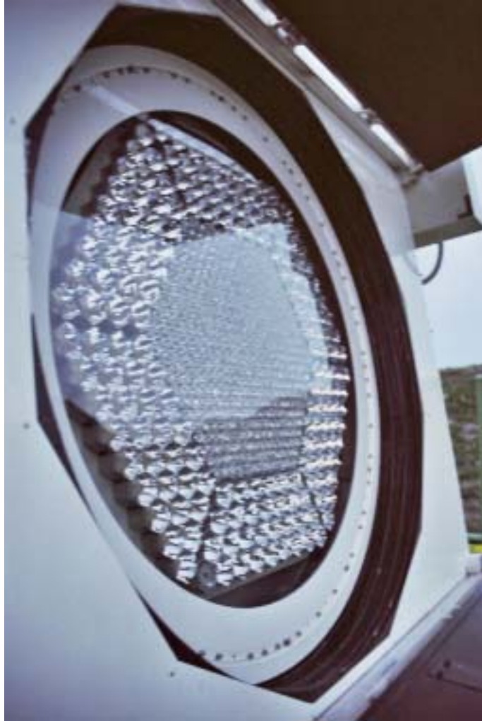
Figure 3.3: Front view image of the MAGIC camera installed in the Telescope frame at La Palma. The plexiglas cover and the light concentrators, which collect the light to the PMT photocatodes, can be seen.
