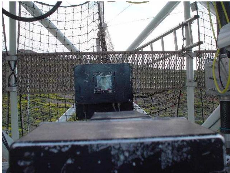
Figure 62: The LED pulser box, seen from the direction of the camera.
