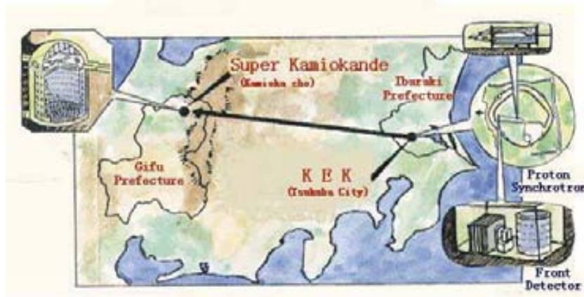
Figure 3.1: Schematic view of K2K experiment placement. Neutrino beam is produced at KEK site and sent to Super-Kamiokande. Neutrinos are detected 250 km from the production point.
