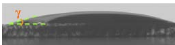
Fig. 3-10: Picture showing the wetting of a 0.003 M BZO-precursor solution on a (001)STO single-crystal substrate.
