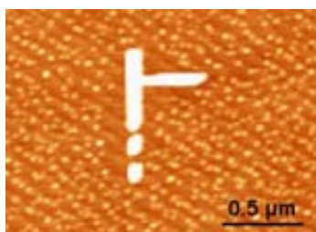
Fig. 5-43: AFM topographic image of a CGO/LAO template with wires and nanodots. Notice the nanodots' void surrounding the wires, illustrating the tendency of (011)-wires to absorb (001)-dots.
