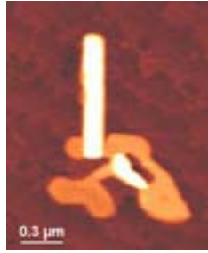
Fig. 5-31: AFM image in the precise moment when the reconstruction of two impinging nanowires takes place.
