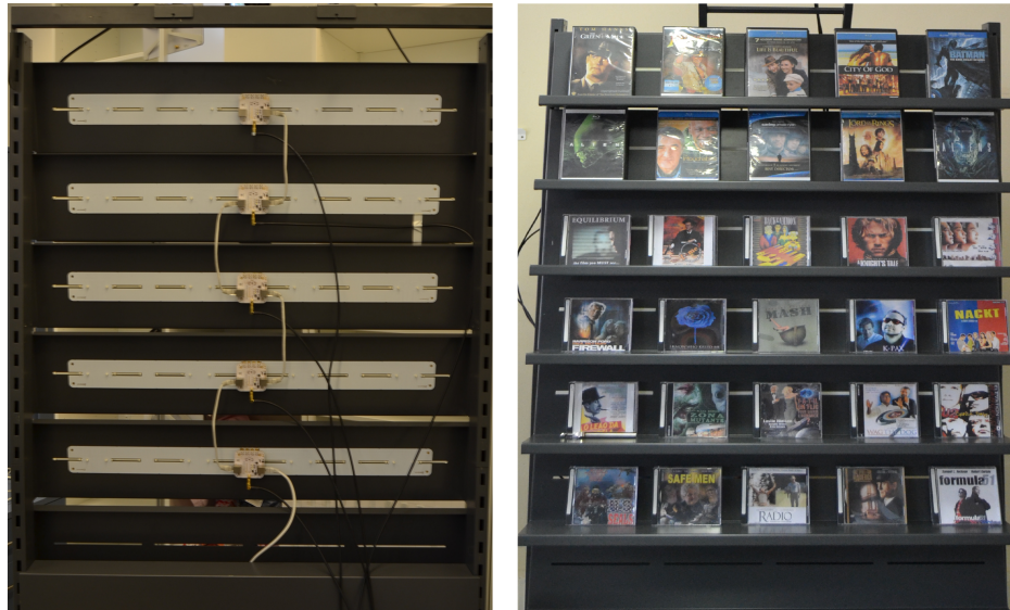
Figure 9.4: A) Back of a Smart Shelf showing the RFID System. B) Frontal view of Shelf with RFID tagged products.
