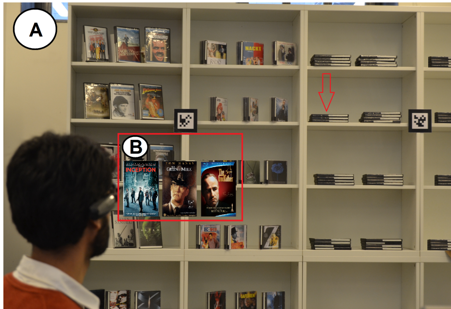
Figure 8.8: A: User is aiming at particular point highlighted with red arrow on the shelves with Smart Glass AR app for a 3 Seconds. B: The items present at user clicked location are shown on the Smart Glass as superimposed images with product information.
