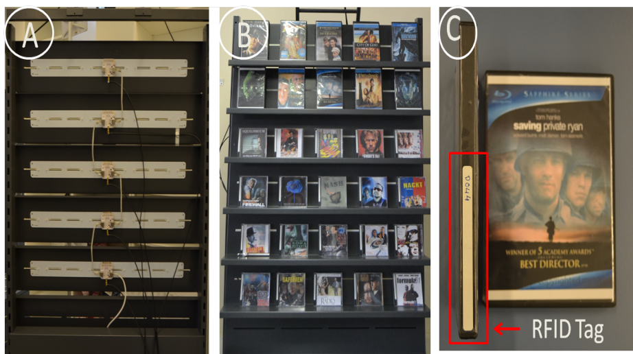
Figure 5.6: A) Back of a Metallic Smart Shelf showing the RFID System. B) Frontal view of Shelf with RFID tagged products. C) Product showing RFID Tag.
