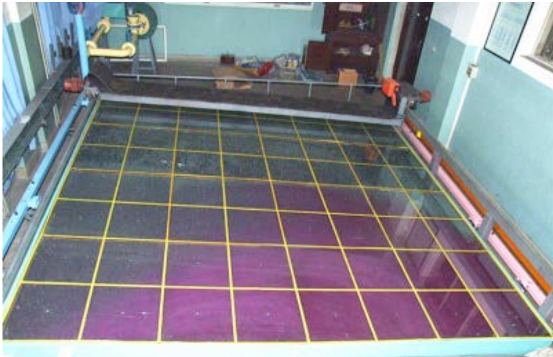
Figure 5.4.2 Gas movement in U-type ventilation system
