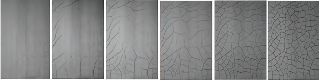
Figure A.5: Sequence showing crack development from appearance of the first crack to the completion of drying and crack pattern formation corresponding to test A0-20
