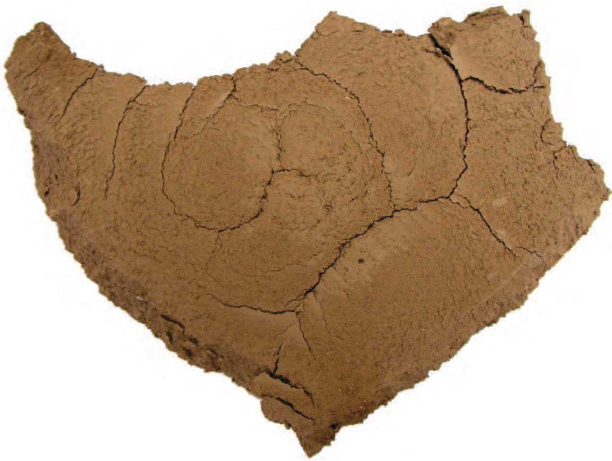
Figure 8.30: Bottom view of cracked polygon 2 from specimen 80-10-P (figure 7.33)
