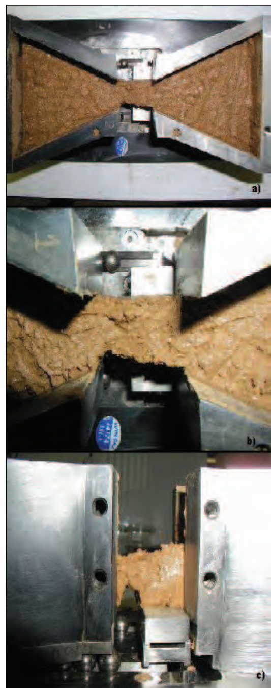
Figure 4.17: Test with constant natural density with moisture content of 30%; (a) plan view of the specimen just after the loading, (b) Zoom of the central part, and (c) side view after failure
