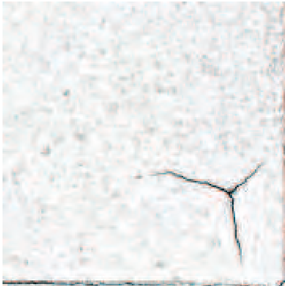
Figure 8.17: Junction formation during the crack nucleation in specimen A2-10
