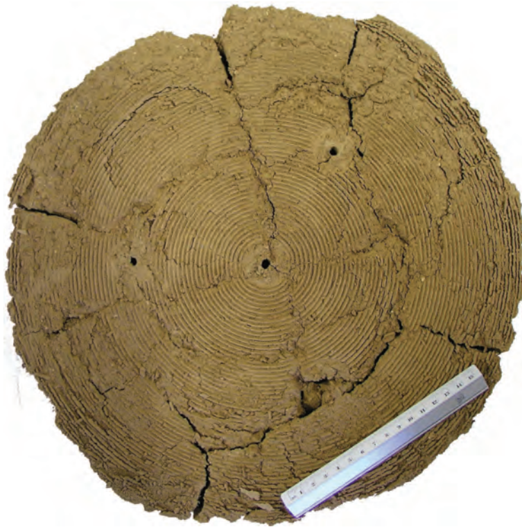
Figure 7.18: Bottom surface of the specimen 40-10 at the end of the test under open laboratory conditions
