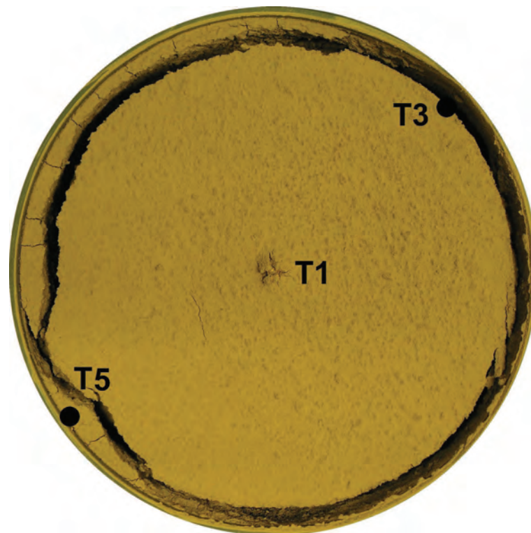
Figure 7.20: Upper surface of the specimen 20-5 at the end of the test under open laboratory conditions
