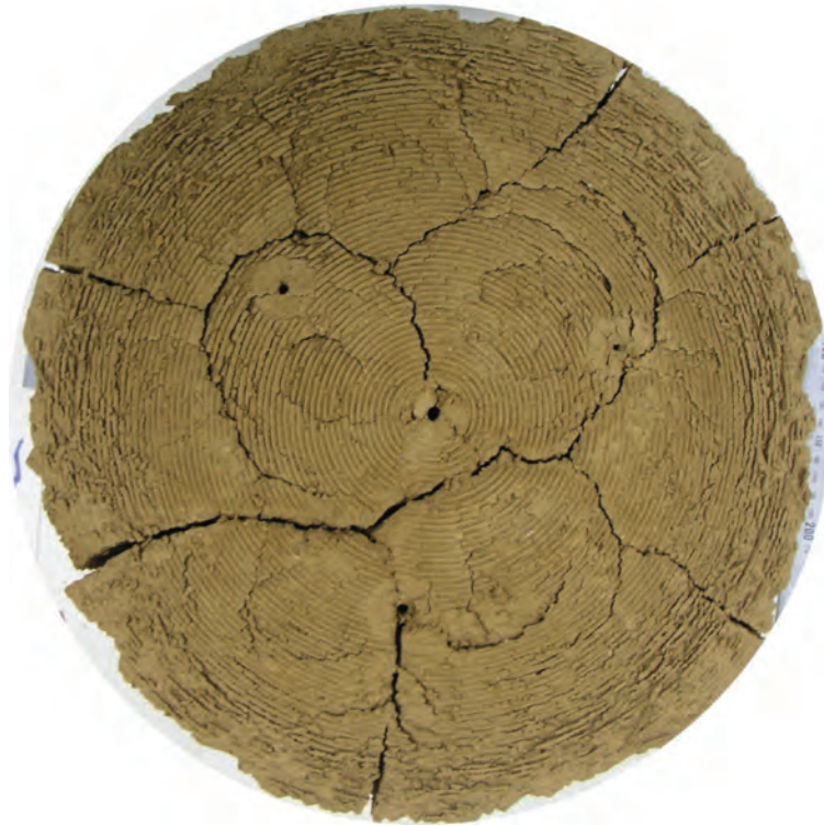
Figure 7.24: Bottom surface of specimen 40-10 at the end of the test carried out in the environmental chamber
