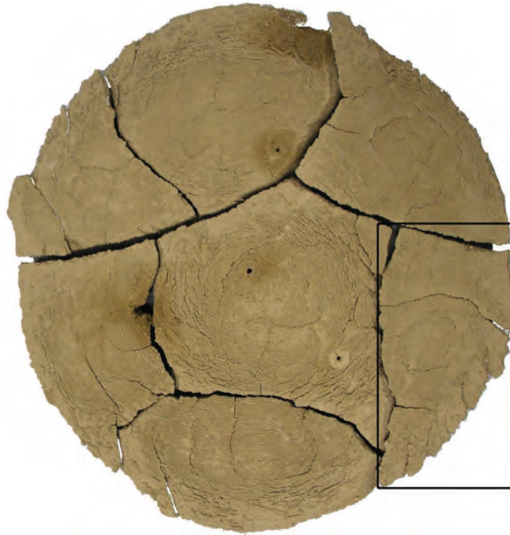
Figure 7.27: Bottom surface of the specimen 80-10 at the end of the test carried out in the environmental chamber
