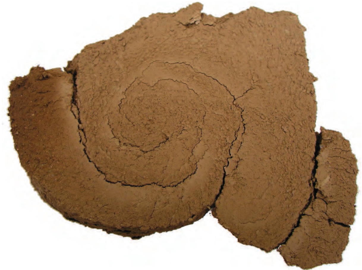
Figure 8.29: Bottom view of cracked polygon 1 from specimen 80-10-P (figure 7.32)
