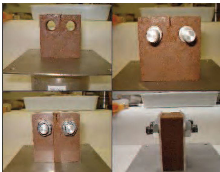
Figure 4.44: Photograph showing the insertion of loading pins and methacrylate plates
