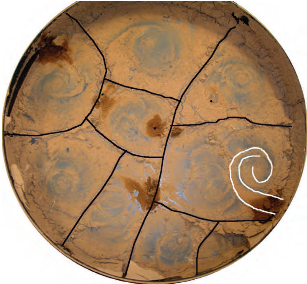
Figure 8.31: Surface of the holding tray with smooth bottom showing the paths left by the cracks and fissures, the image was taken at the end of test 80-10-P after careful removal of the cracked cells. The black lines correspond to the cracks which were seen in the top and bottom and the white line correspond to the spiral cracks observed only at the bottom.
