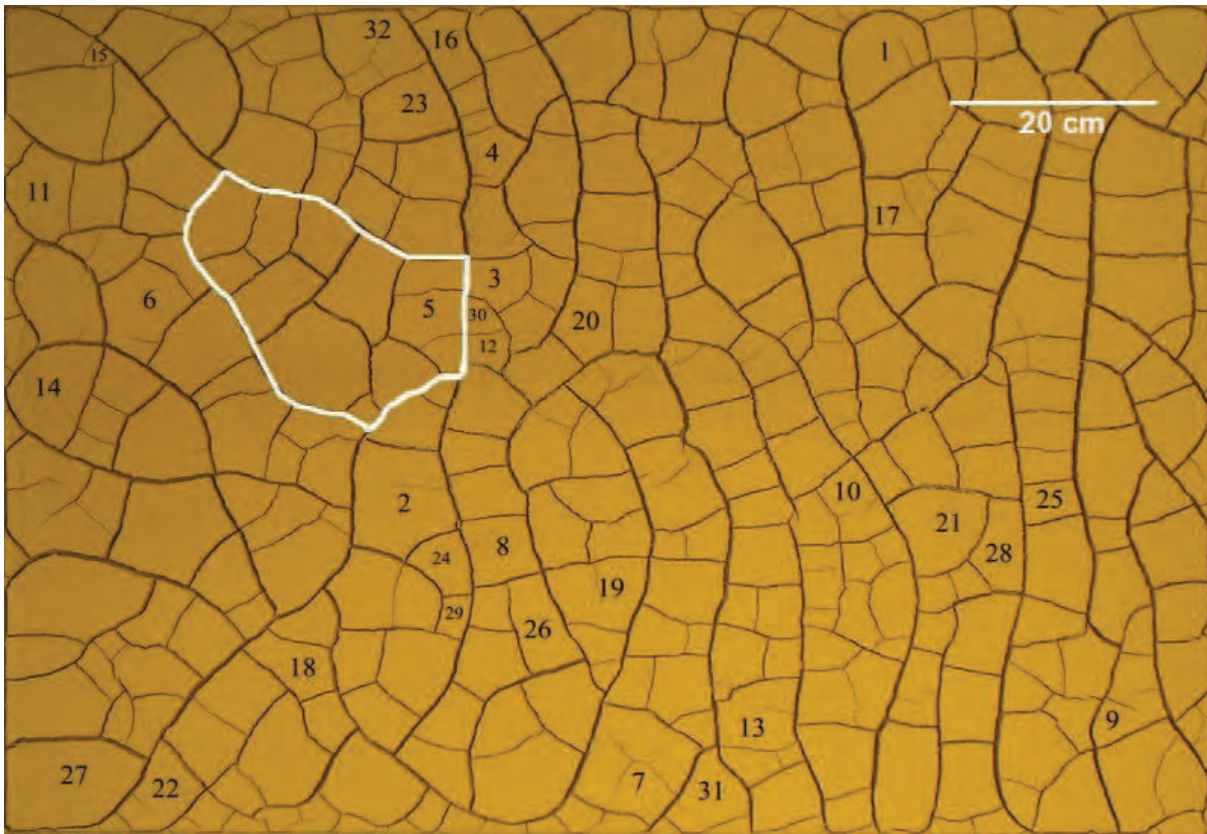
Figure 8.2: Final crack pattern on specimen A0-20. The numbers indicate the cracked polygons selected for further detailed analysis and the white border marks the area selected for monitoring of its time evolution.
