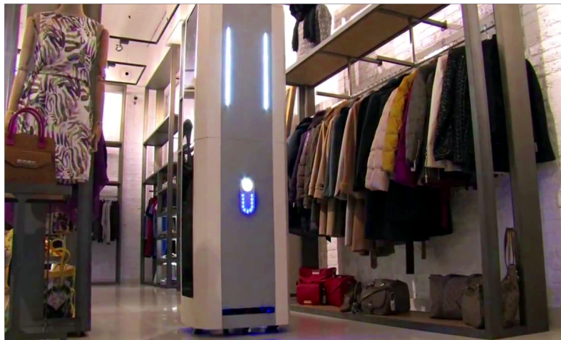
Figure 3.6: AdvanRobot is reading RFID tags and their approximate locations by going around the retail store.
