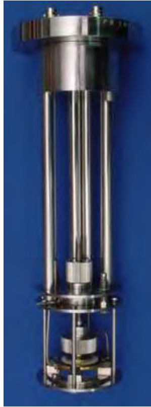
Figure 3.6: The parallel plate electrodes BDS 1200. The figure was taken from [57]
