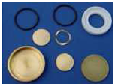
Figure 3.7: The Liquid Sample Cell BDS 1308. The figure was taken from [57]
