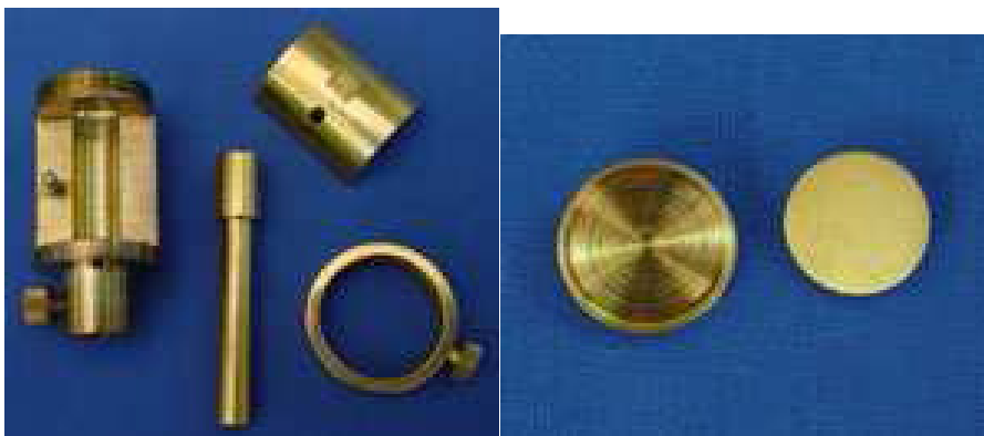
Figure 3.10: The RF Liquid Sample Cell BDS 2200. The figure was taken from [57]
