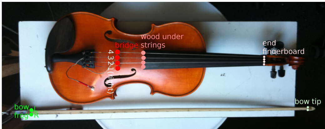
Figure 3.5: Detail of the marked string and bow ribbon positions relative to the wired motion capture sensors used for the acquisition of instrumental gestures.
