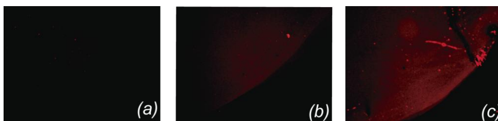
Figure 2. 37 Fluorescent signals after the incubation of the SH-DNA probe with different sulfo-GMBS crosslinker concentrations: (a) 5, (b) 10 and (c) 20 \mu\text{M} previously to surface biofunctionalization.
