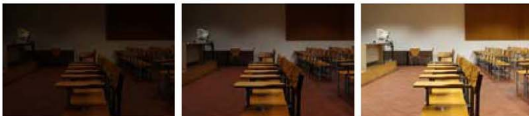
Fig. 3 Three standard scenes on Experiment 1, with average illuminance levels of 1, 7.5 and 530 lux over the working surface
