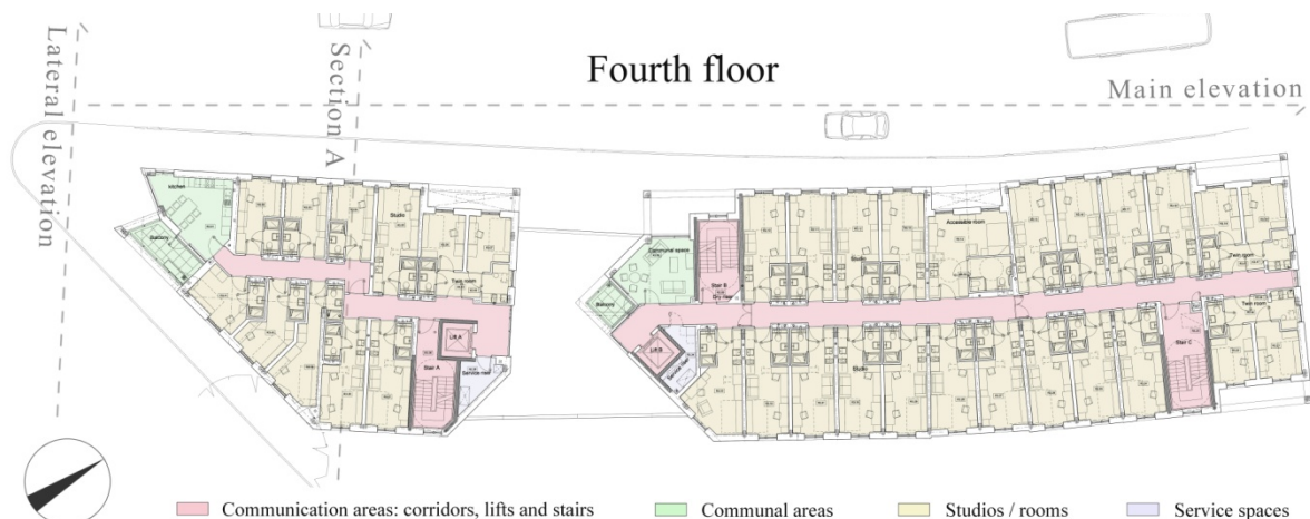
Fourth (and type) floor of the Urban Nest student residential building.
