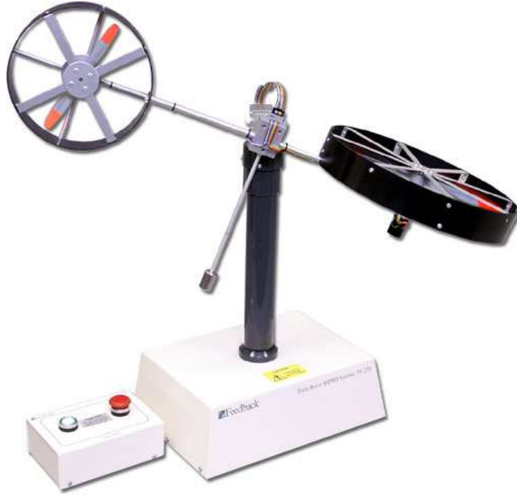
FIGURE 8.3: Twin rotor MIMO system (TRMS).
