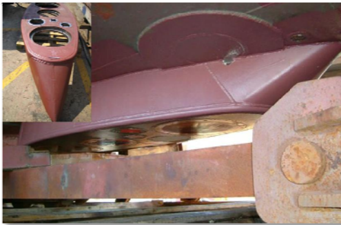
Figure 1.4. Protruding keel installed at the hull of the R/V Cornide de Saavedra in 2006 (image by Joan Miquel Batle).
