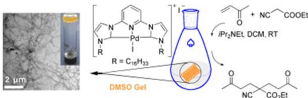
Figure 9. Macroscopic and microscopic structure of the Palladium Pincer complex and its application as catalyst in a double Michael addition reaction. 36
