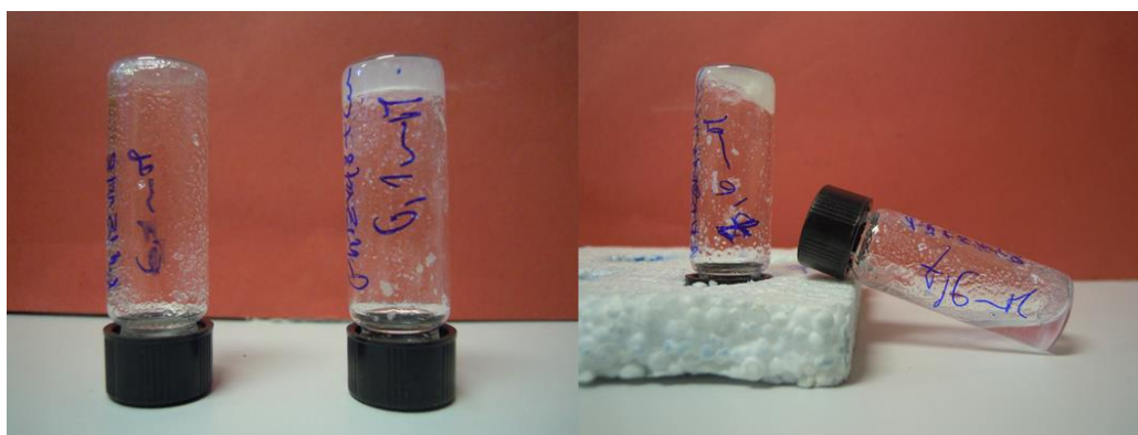
Figure 27. Macroscopic aspect of the PhTzVal 8 gels of the corresponding metallo gels at concentrations of 6.1 mM and 7.6 mM, 24h after their disintegration in the T_{sol} determination experiment.
