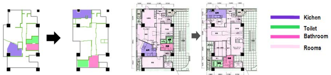
Figure 36: NEXT 21 dwelling transformation: Transformations of the mayor functional end technical systems: façade perimeter, façade cladding, kitchen and bathroom position, partition walls changing position
