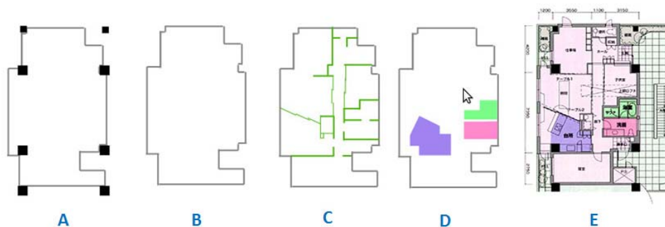
Figure 37:: Next 21: Independent subsystems at the dwelling level: A - load-bearing module; B - envelope cladding, doors and windows; C - interior partitions, fittings, interior finishes, the doors and windows; D - dwellings' services: ducts, pipes, and wirings.; E - equipment, furniture. (Appendix - NEXT 21 Open Building experimental project)
