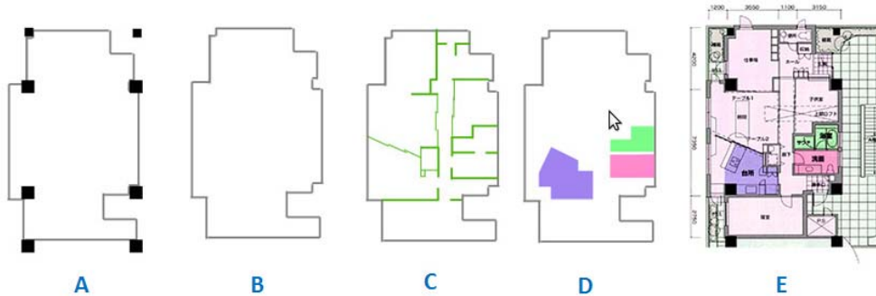
Figure 12: Next21: Subsystem at the “infill” level: A - Structural module; B - Unit cladding, doors and windows; C - Interior partitions, fittings, interior finishes, the doors and windows; D - Dwelling services / (ducts, pipes, and wiring of mechanical systems are placed in floor or ceiling spaces, which allow flexibility for the location of kitchens and bathrooms in dwelling units.; E - Equipment, furniture.
