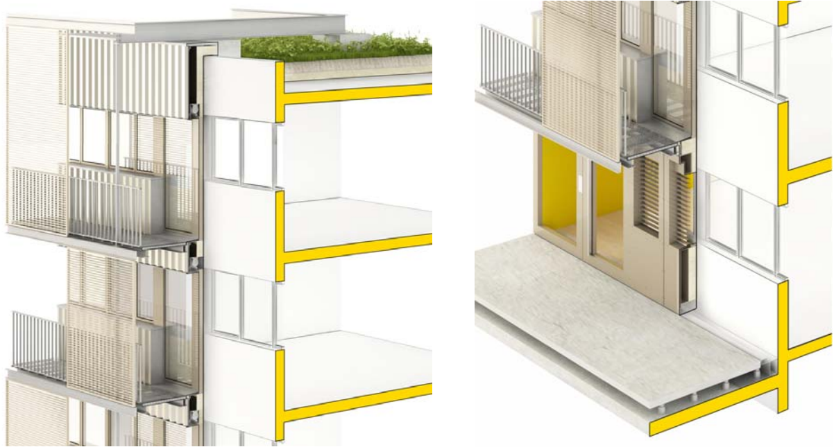
Figure 17: System for new industrialized façade system
