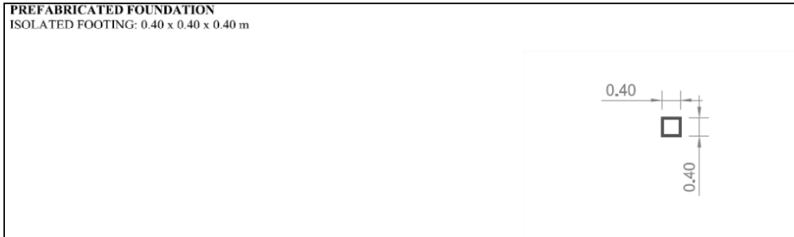
Figure 141. Precast foundation under analysis: dimensions and plan.
