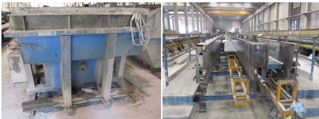
Figure 1. Precast isolated footing mold. Figure 2. Precast beam mold.
