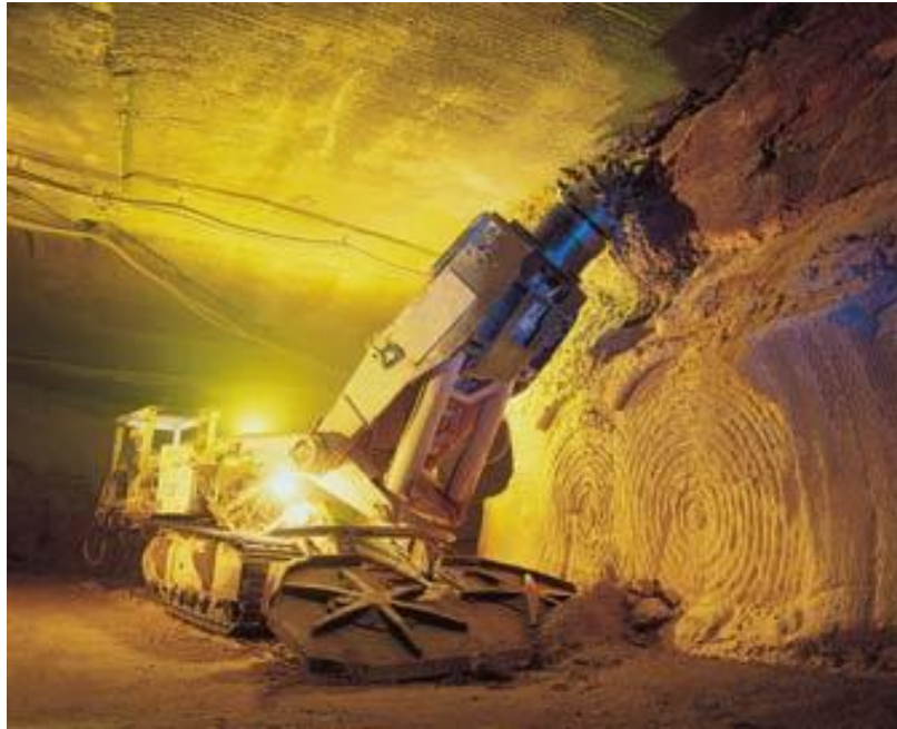
Figure 5. Axial continuous mining machine (Source: Mineral resources of Saskatchewan).
