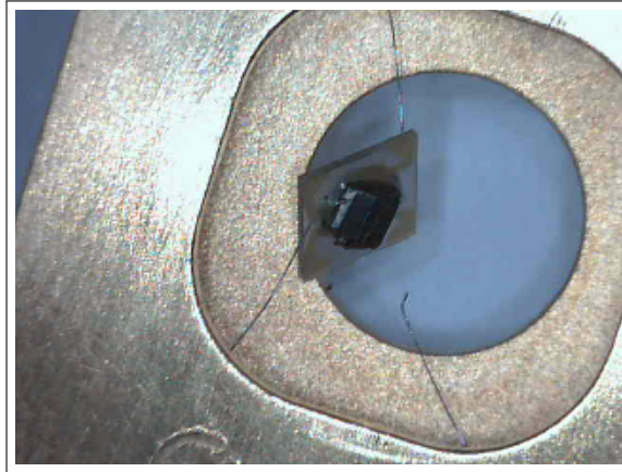
Figure 5.12: The calorimeter after the magnetic torque break the connecting wires of the platform.
