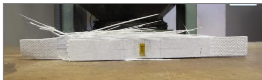
Figure A.9: Tensile failure of specimen W1 in the proximity of one of the action grips.
