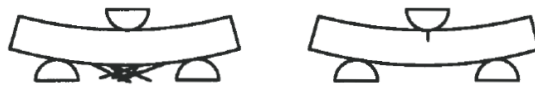
Figure A.4: Tensile fracture and compression fracture of fibers due to flexure [155].
