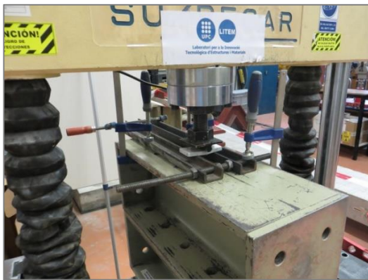
Figure A.33: Test setup configuration for interlaminar shear tests.
