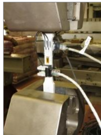
Figure A.12: Tensile GFRP specimen positioned in the action grips.
