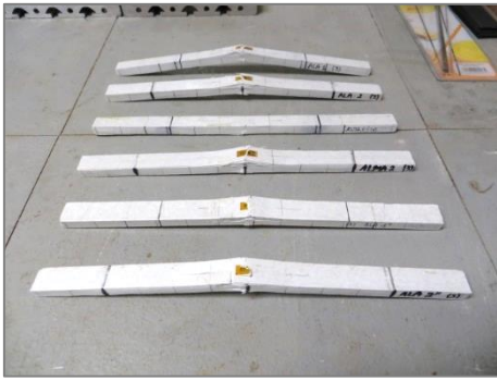
Figure A.5: Bottom-up view of the flexural failure of the GFRP specimens.
