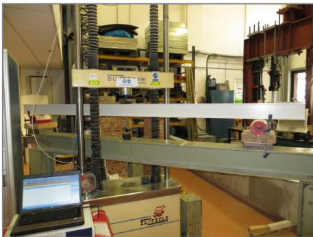
Figure A.47: Profile bending setup for a test span of 2500 mm.
