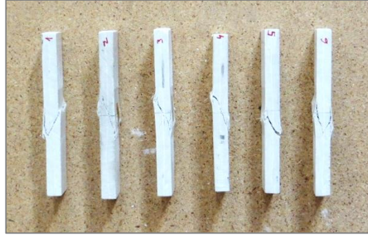
Figure A.26: Compressive failure of the GFRP crosswise specimens.
