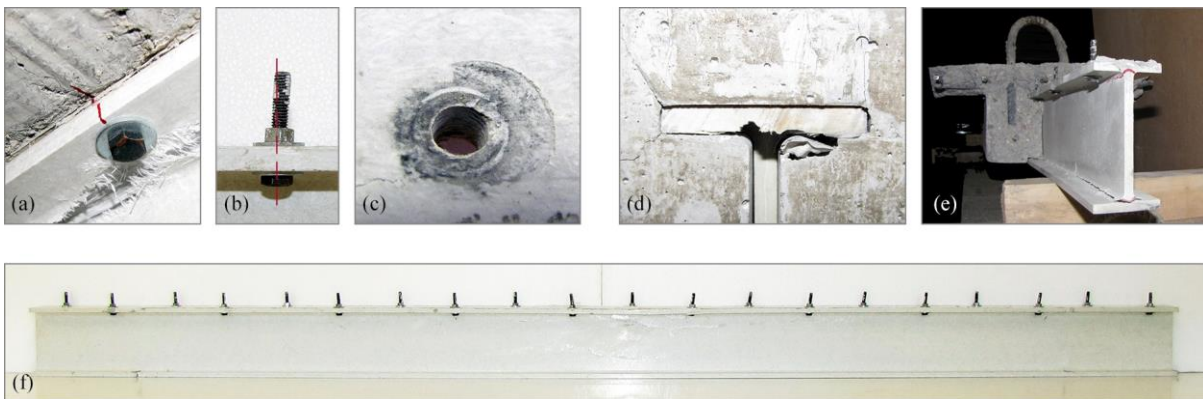
Figure 3.48: Visual evidence of partial shear interaction and shear failure: (a) occurrence of slip and junction shear; (b) deformation of bolts; (c) distortion of connector holes; (d) web-flange rupture; (e) top and bottom flange delaminations of M1-HB2; (f) radial inclination of bolts in M2-HB2 (concrete slab removed).
