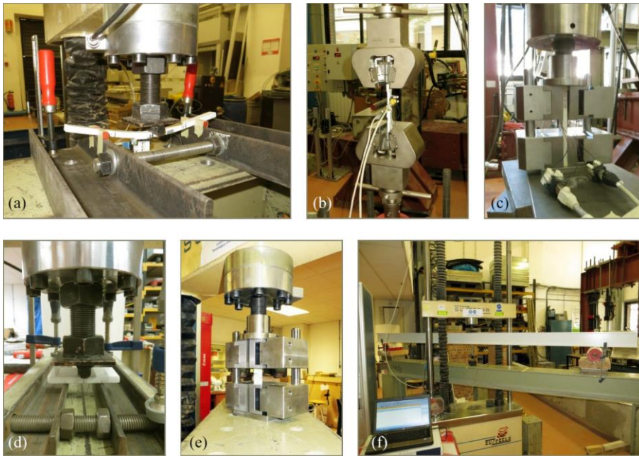
Figure 3.6: GFRP profile material characterization tests: (a) flexure; (b) tension; (c) in-plane compression; (d) interlaminar shear; (e) in-plane shear; (f) full section effective moduli.
