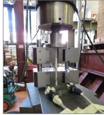
Figure A.21: Experimental test setup configuration for compressive tests.
