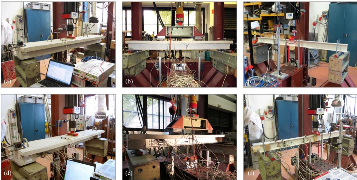
Figure 3.26: Laboratory setups and instrumentation: (a) M1 or M0 beams in test setup I; (b) M1 or M0 beams in test setup II; (c) Profile 1 in test setup I; (d) M2 beams in test setup I; (e) M2 beams in test setup II; (f) Profile 2 in test setup I.
