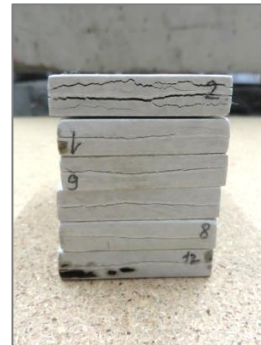
Figure A.37: Lateral view of the interlaminar shear failure of all coupons.
