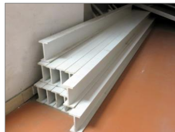
Figure 3.2: GFRP profiles used in the experimental campaign.
