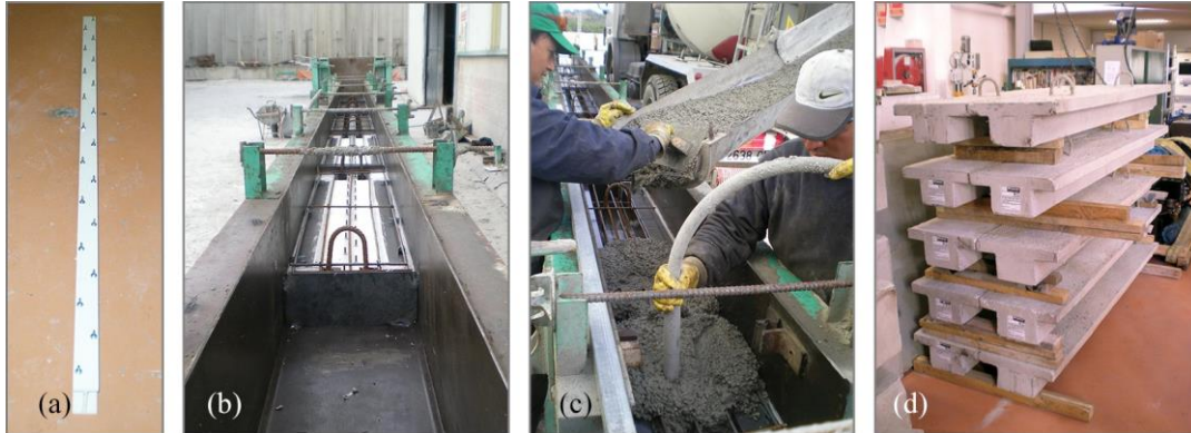
Figure 3.8: Fabrication process of the hybrid beams: (a) installment of steel bolts; (b) completed formwork; (c) concrete casting; (d) specimens prior to instrumentation and testing.
