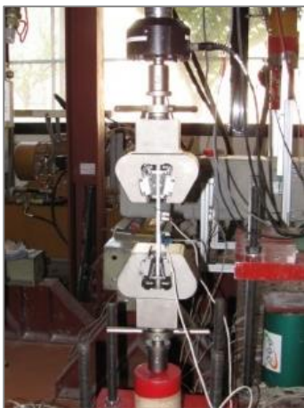
Figure A.11: Experimental test setup configuration for tensile characterization tests.
