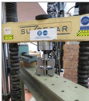
Figure A.41: Test setup configuration for in-plane shear tests.
