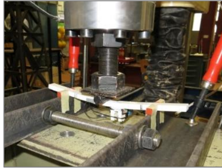
Figure A.3: Experimental test setup configuration for flexural characterization tests.
