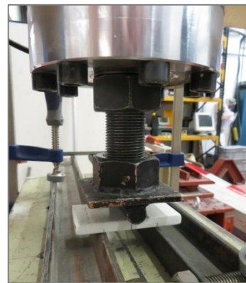
Figure A.34: Loading and support arrangement for interlaminar shear tests.
