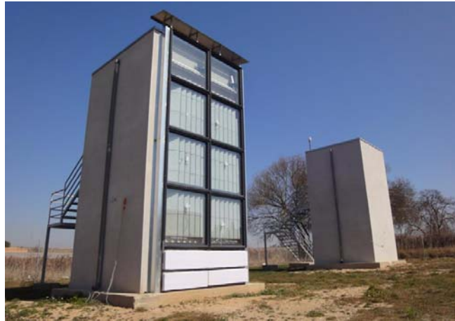
Figure 5. Double skin facade with PCM (left) and double height reference cubicle (right)
