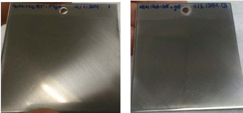
Figure 4. 48 - Images of 76M:14G:10T+0,9wt.%gel (left) and 56M:14G:30T+0,9wt.%gel (right) biocoatings on stainless steel plates.
