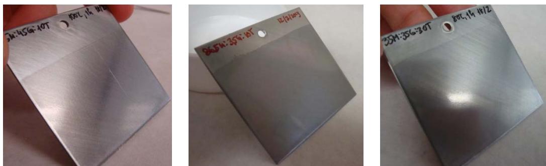
Figure 4.10 - Images of some biomaterials coated on stainless steel plates. Material with molar silane composition 45M:45G:10T (left), material with molar silane composition 86,5M:3,5G:10T (center) and material with molar silane composition 35M:35G:30T (right).
