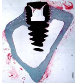
Figure 4.84 - Cross section of coated implants with 50M:50G reference material after 8 weeks healing time (light microscope images 1000X). (reproduced by courtesy of 1 )
