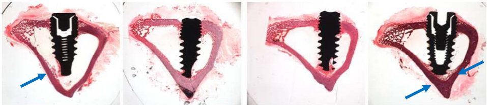
Figure 4. 88 - Cross section of uncoated titanium implants after 2 weeks healing time (light microscope images 1000X). (reproduced by courtesy of 1 )
