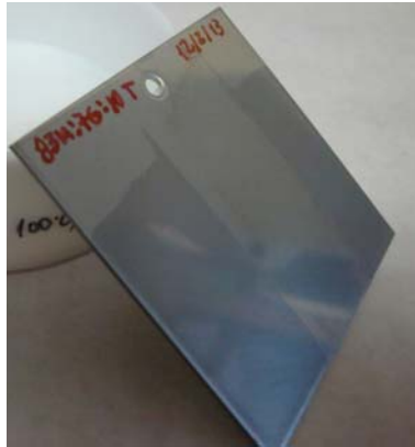
Figure 4.22 - Prepared sample for average roughness ( R_a ) measurement of 83M:7G:10T biocoating.
