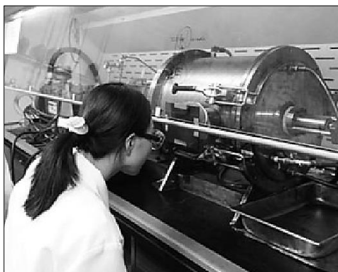
Figure 1.3 Krätzschmer-Huffman arc reactor for the synthesis of fullerenes. Photography published 37 by the Echegoyen's research group.
