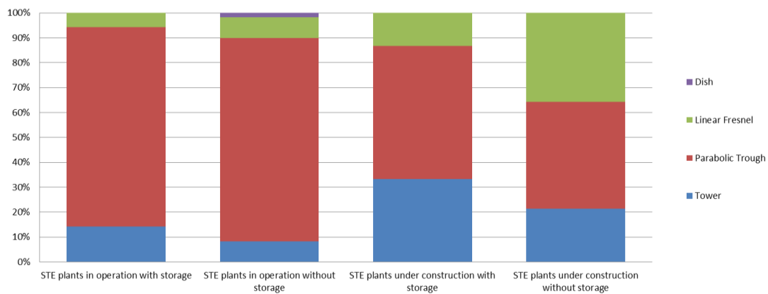
Figure 4. STE worldwide capacity categorized by technology and with/without storage (January 2016) [9]
