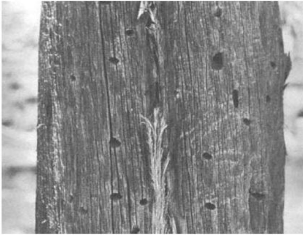
Figure 10 Beetle exit on a juniper fencepost, near St. John's, Arizona (from Schiffer 1987: 198, Figure 7.9).
