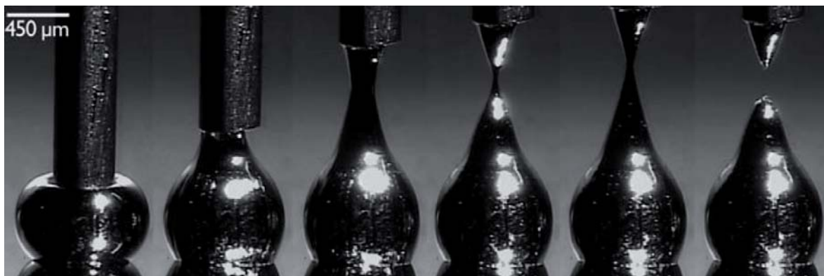
Figure 21: A sequence of images to show the formation of the EGaIn conical tip. 85
