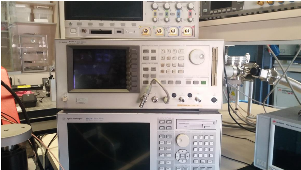
Analizador de redes: AGILENT E5100A Network Analyzer (10kHz-180MHz)
