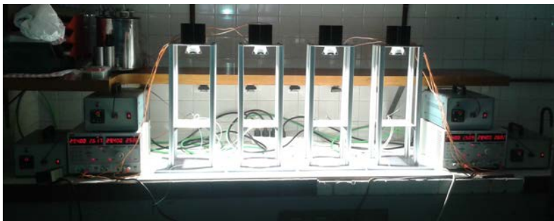
Figure 2.8: Photography of the operating solar cell illuminator.
