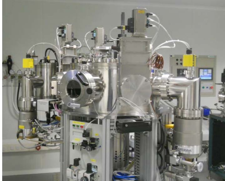
Figure 2.1: Photography of the PECVD reactor in the cleanroom of the Universitat de Barcelona (before the HWCVD chamber installation.)
