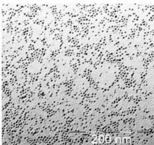
Figure S1. TEM micrograph of spherical Pd NPs.
