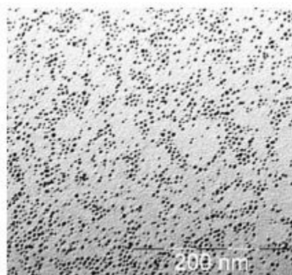
Figure 5.9. TEM micrograph of spherical Pd NPs
