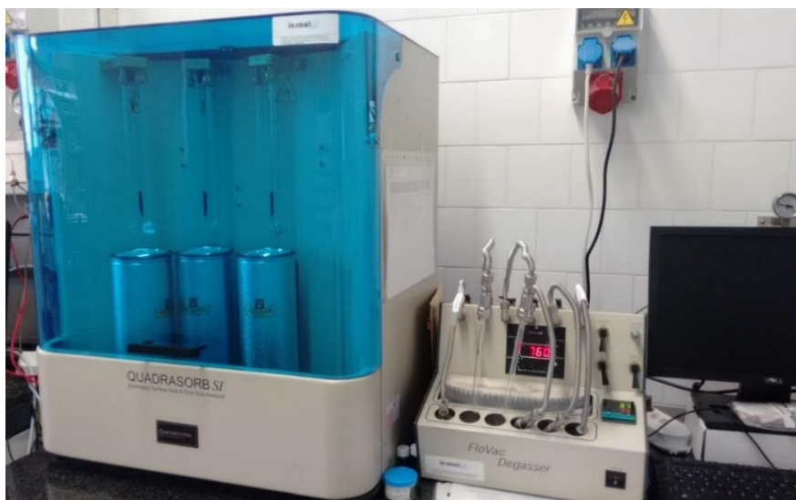
Figure 2.5. N 2 -physisorption equipment
