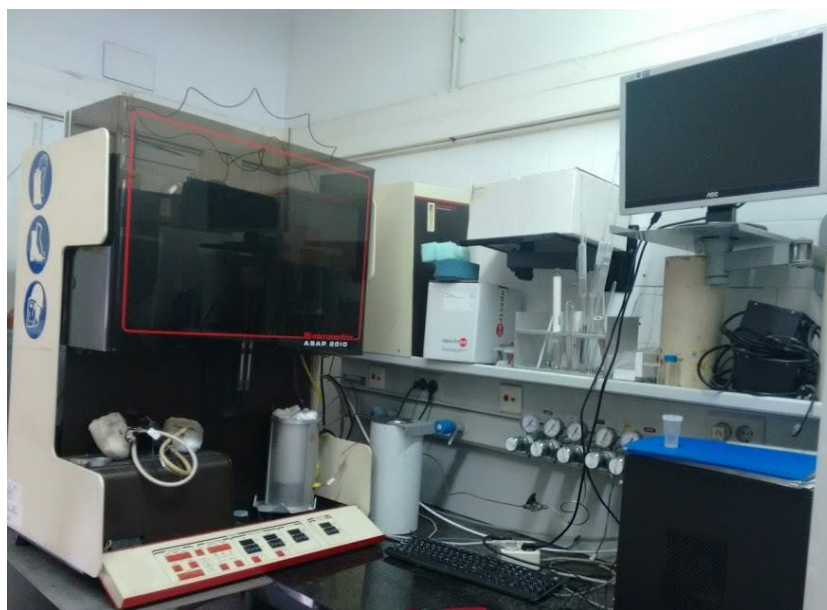
Figure 2.15. H 2 -Chemisorption equipment
