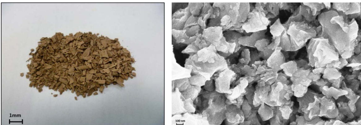
Fig. 3.2 Prepared catalyst (left hand side) and its microscopic picture (SEM) (right hand side)
