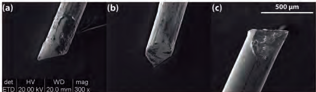
Figure C.3: FE-SEM images of different Ni STM tips used to perform STM-BJ experiments.
