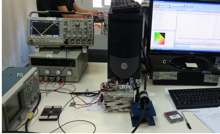
Figure 6.16: Experimental set-up to characterize laser under CWFM-OF . OSC: oscilloscope, PS: power supply, FG: function generator, SM: spectrometer, C: computer, T: stationary target, BS: beam splitter, L: lens, LD: laser diode, PD: photo-diode, DR: driver and modulator.
