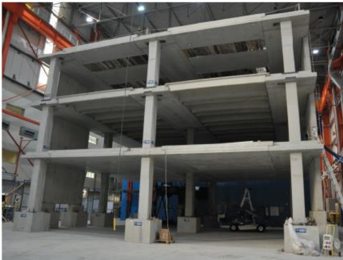
Figure 5.12. The structural prototype.
