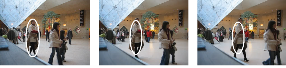
Figure 2.2: Example of a color-based particle filter for people tracking.
